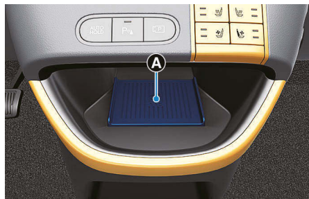
[A] Vehicle authentication pad (Wireless charging pad)
