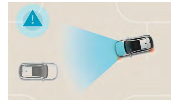
Forward Collision-Avoidance Assist with Junction Turning (FCA-JT).
