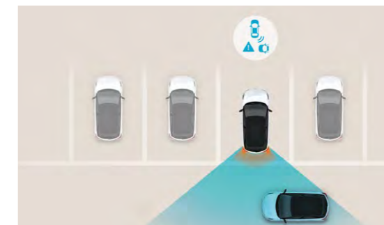
Rear Cross-traffic Collision-avoidance Assist (RCCA).
